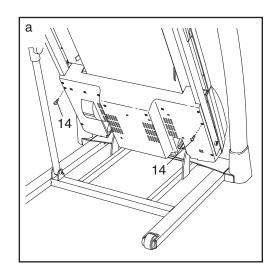
Remove the four #8 x 3/4" Screws (14) and carefully remove the Motor Hood (61).
